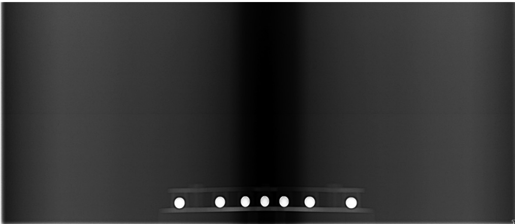
Fig. ⑧ -62: Steel balls spread in the Y direction (distances between steel balls meet benchmark)
