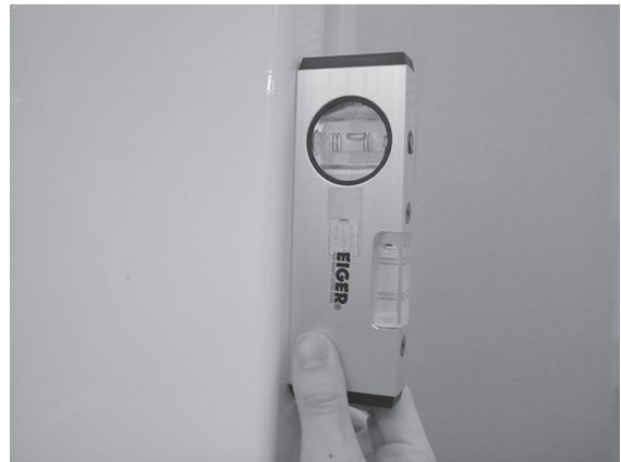
Fig. ③ -27: Checking for column lean
