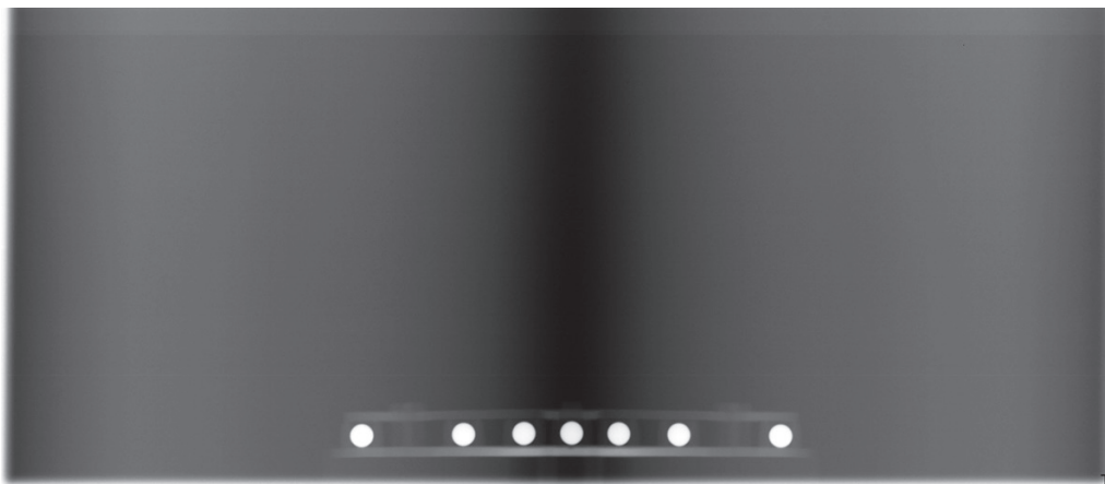
Fig. ⑧ -60: Captured Installation phantom image
