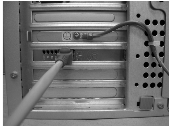
Fig. ④ -37 : Protective grounding wire connection
