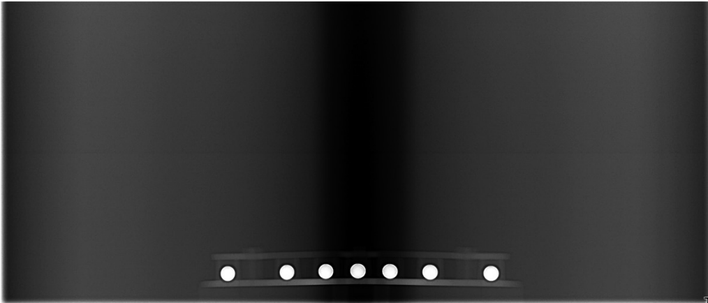
Fig. ⑧ -61: Steel balls spread in the X direction (distances between steel balls meet benchmark)
