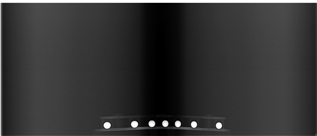
Fig. ⑧ -63: Distances between steel balls incorrect (distances between steel balls do not meet benchmark)
