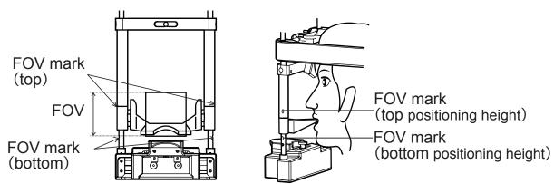
Note : Do not align the up-down positioning height while the lock lever is in locked condition. This may cause failure.
