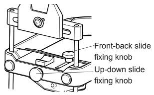
The forehead support can slide vertically if the up-down slide fixing knob is loosened. Position the forehead support at the height of the patient's head, and tighten the updown slide fixing knob.
