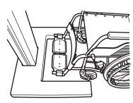
When an optional normal-sized base is used, position the wheelchair so that the front wheels sit nicely between the base and rear wheels are free from hitting the base.
