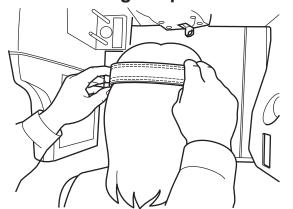
Position the patient's forehead at the forehead support, and stabilize the patient's head by using the head band. At that time, ask the patient not to lean on the head fixator for 3D image acquisition.
