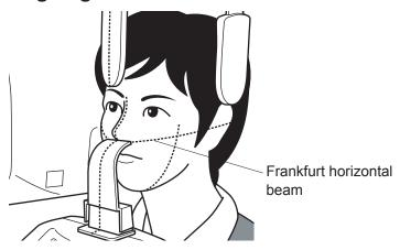
Align the horizontal line of the head support parallel to the camper plane on patient's head. Moves the sliding mechanism up or down to adjust the chin rest height so that the TMJ adaptor may be positioned at the subnasal point. Then, make a fine-adjustment to align the Frankfurt horizontal beam to the camper plane on the patient's head.
