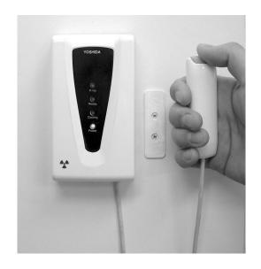
Make sure that the Ready LED (green) is turned on and the equipment is ready for image acquisition. Press the X-ray Exposure switch to start image acquisition. Holding down the switch activates X-ray Exposure during the specified Exposure time. While Xray is irradiated, the X-ray indicator (yellow) on the hand-switch box turns on, and the buzzer continually buzzes. An audible alarm also sounds at the control panel.
