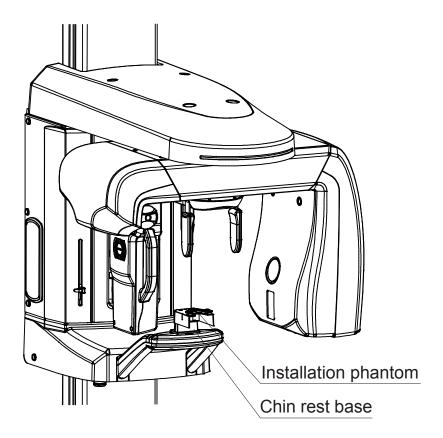
Acquire image of the Installation phantom under the following conditions.
