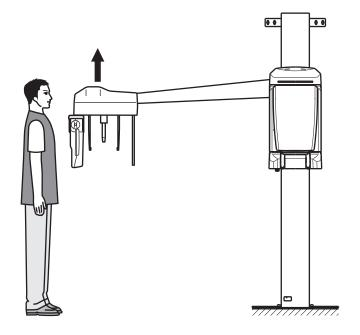
Press the Reset Switch on the Control Panel. The arm unit and sensor unit automatically move to the Cephalometric image acquisition position, and the slits in the head unit automatically switch.
