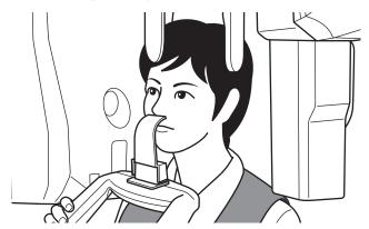
Ask the patient to close their mouth. Check that the patient has closed their mouth and then press and hold down the X-ray Exposure switch until image acquisition is successfully finished. To scan images of left and right temporomandibular joints, total of 8-second X-ray exposure is executed on both joints, 4 seconds each. After X-ray exposure, release your finger from the X-ray Exposure switch.
