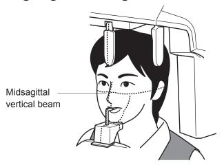
Once the patient has been positioned inside the equipment, press the Positioning beam switch. The rotating arm unit will move to the positioning point and the beam will be emitted. Then, align the midsagittal vertical beam to the patient's midsagittal line. Check in the positioning mirror that the beam is right on the patient's midsagittal line. (The correct line runs through the middle point between the left and right incisors and the nose ridge.)
