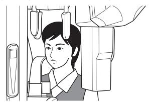
Set the chin rest at the height of the patient's jaw. Position the patient inside the equipment and moves the sliding mechanism up or down on the control panel so that the TMJ adaptor is positioned at the patient subnasal point with the back straighten up. Then, press the Beam switch to activate the positioning beam.
