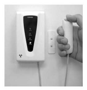
Make sure that the Ready LED (green) is turned on and the equipment is ready for image acquisition. Press the X-ray exposure switch to begin the X-ray radiography. By holding the X-ray exposure switch down, X-ray is irradiated according to the acquisition time specified. While X-ray is being irradiated, the X-ray LED (yellow) on the hand-switch box is lit and buzzer on the Control Panel goes off continuously.
