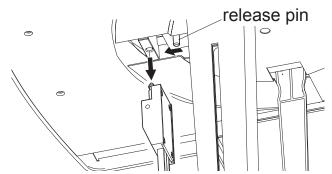
As shown on the picture on the left, pull the release pin of the nose support for detachment.
