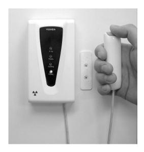
Make sure that the Ready LED (green) is turned on and the equipment is ready for image acquisition. Press the X-ray exposure switch to begin X-ray radiography. By holding the X-ray exposure switch down, X-ray is irradiated according to the acquisition time specified. While X-ray is being irradiated, the X-ray LED (yellow) on the hand-switch box is lit and a buzzer sounds continuously. It also sounds from the Control Panel.
