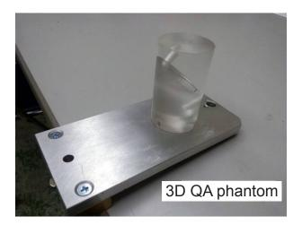
Attach the 3D QA phantom to the chin rest base. Conduct image acquisition in two modes, Dental Mode and Oral Mode.
