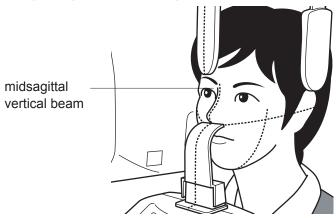
After Position the patient inside the equipment, press the Beam switch. The rotating arm unit moves to the positioning point and the positioning beam activates.
