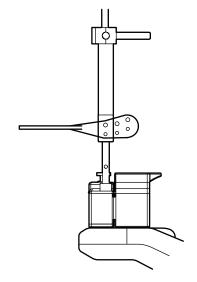
For wisdom teeth image acquisition, insert the front row pins of the bite plate to attach.
