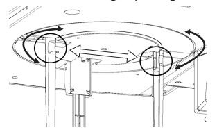
Hold the indentations pictured left and rotate the nose support and ear rods.
