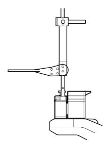
1 For front teeth image acquisition, insert the rear row pins of the bite plate to attach.
