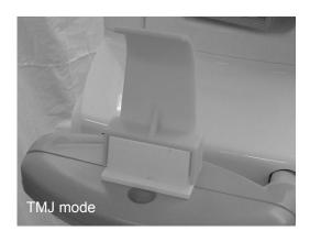
Remove the chin rest and attach the TMJ adaptor to the chin rest block base.
