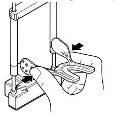
Coat the bite plate with dental impression material (Use general commercial products, "dental alginate impression materials", "Dental Silicone impression materials", etc). Advise the patient to bite on the bite plate coated with dental impression material. Wait until the impression material hardens.
