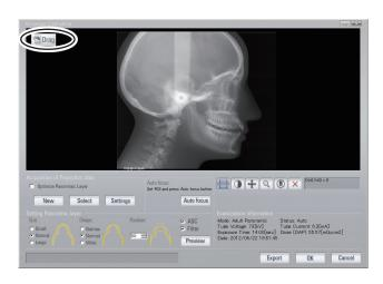
When X-ray irradiation is initiated, the equipment starts transferring the image data to the computer (Image Creator). Once the transfer is complete, Image Creator starts formulating and displaying the cephalometric image.
