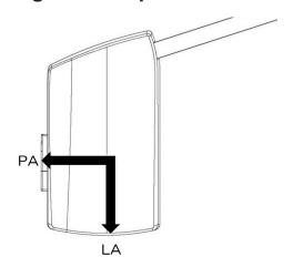
Turn the ear rod and nose support of the Cephalometric Unit to the appropriate position according to the desired image acquisition mode, namely "Posteroanterior Image (PA)" or "Lateral Image (LA)". (The arrow indicates the direction of which the patient should face.)
