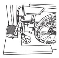
When an optional wide base is used, fold up the foot rests of the wheelchair if necessary in order to position the wheelchair all the way to the column.
