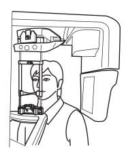
Seat the patient and move the chin rest unit up and down to adjust the bite plate to the height of patient's mouth. Press the Up/ Down switch on the control panel to move the chin rest unit up and down.
