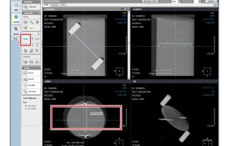
Adjust the tilt of the crossbar, and measure the distance between the two steel balls.
