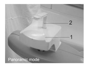
Insert a bite block (2) into the chin rest block (1).
