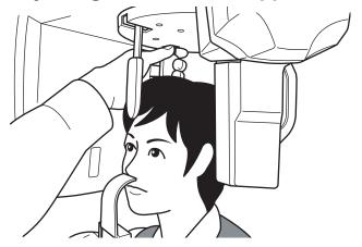
Slide the forehead support in contact with the patient's head by gripping its base and then close it. With the Auto setting, the tube voltage appropriate for the patient is automatically set. At the end of adjustment, turn on the positioning beam again to confirm that the beam is right on the proper point.
