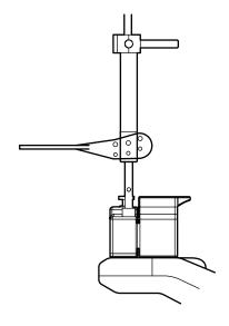
**2** For molar teeth image acquisition or front teeth 3D Oral image acquisition, insert the center row pins of the bite plate to attach.
